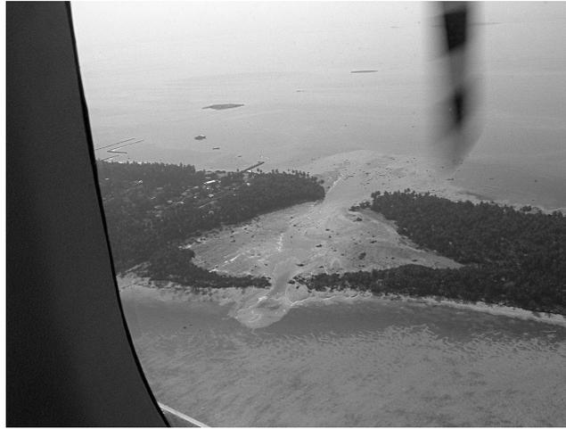
**Figure 9.** Westward view of the Kolhufushi lagoon and the sand spit, which was breached by the tsunami.
