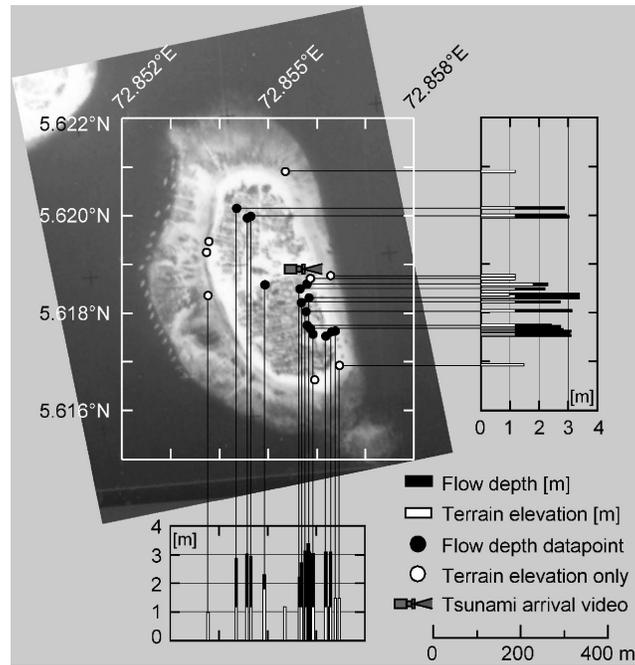
**Figure 11.** Measured tsunami flow depths and surveyed locations at Kandholhudoo, on a pre-tsunami satellite image provided by the Maldives Disaster Management Center.
