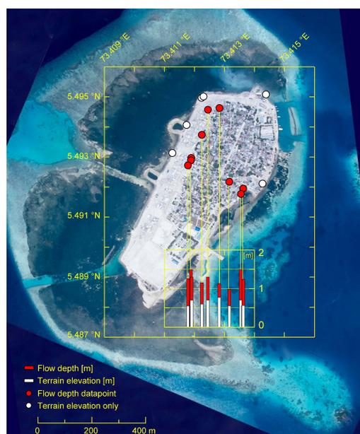
**Figure 13.** Hinnavaru Island (Lhaviyani): measured tsunami flow depths and surveyed locations on a pre-tsunami satellite image provided by the Maldives Disaster Management Center.
