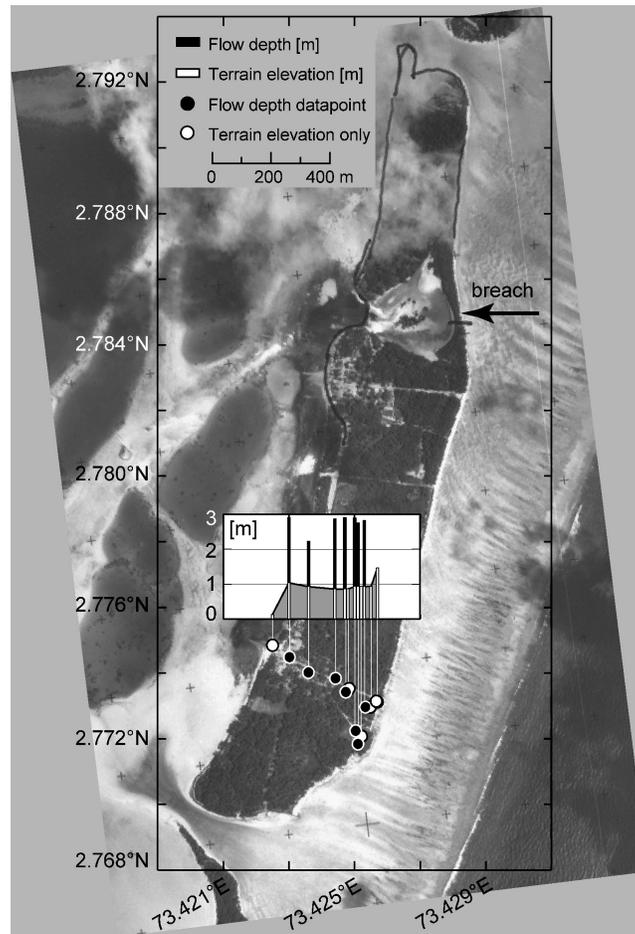
**Figure 8.** Kolhufushi Island (Meemu Atoll): measured tsunami flow depths and surveyed locations. The sand spit connecting the northern end of the island is not breached in this pre-tsunami satellite image provided by the Maldives Disaster Management Center.
