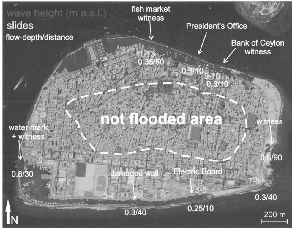
**Figure 2.** Flow depths at several locations around Malé. The interior of the island (inside the dashed line) was not flooded during the tsunami.
