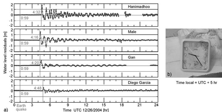
**Figure 7.** Tsunami arrival time: (a) analysis of tide gauge residuals; (b) broken clock recovered on Vilufushi Island.
