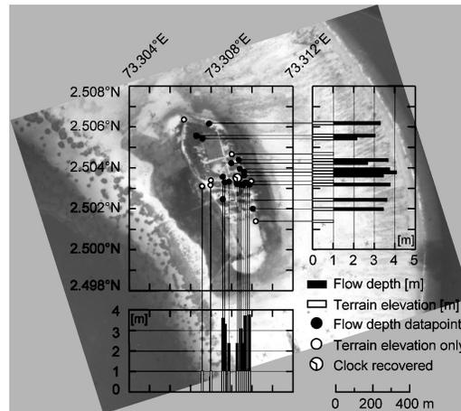
**Figure 6.** Measured tsunami flow depths and surveyed locations at Vilufushi, on a pre-tsunami satellite image provided by the Maldives Disaster Management Center.
