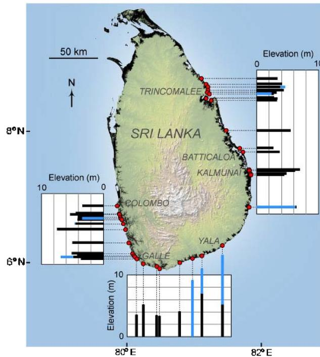
**Figure 1.** Measured tsunami runup (in blue) (in grayscale: gray) and maximum tsunami heights (in black). Red-filled dots (in grayscale: gray) show the sites of elevation measurement; areas shaded in black are less than 10 m above sea level. The map is modified from one by ASTER (after Liu et al. 2005). In the online version of this figure, the measured runup is in blue, and the maximum tsunami heights are in red.
